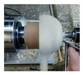
Some off-lathe sanding will be needed to remove the nubs at the bottom, where the drive center was at the end of the cup, and at the end of the handle. Also sand around the edge for a "nice feel" on your mouth.
