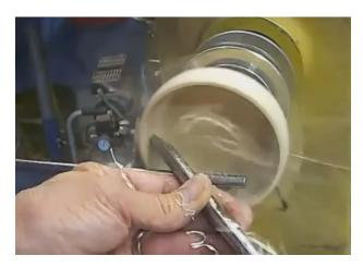
Some light sanding inside the cup is appropriate. Be very careful of that handle if you choose to sand with the lathe running. Much safer to hand sand or power sand with a 2" disk, with the lathe stopped. You don't need a perfect surface - 120 or 180 grit should be sufficient.
