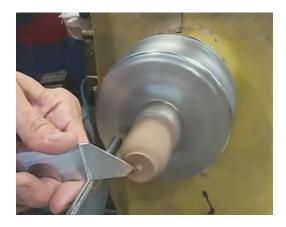
Jam the button on the spigot. If your jam chuck is a bit loose, add a bit of paper towel to make it snugger.
