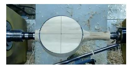
You can do some sanding on the handle now, but be very careful of the off-center cup. You really can't sand the cup while it's spinning, so sand that off the lathe. I usually sand very little as the tool marks sort of prove that I turned it - maybe just a light pass with 120. This is an "outdoorsy" piece, intended to be used (and abused), so a somewhat rugged look is appropriate.
