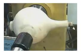
Watch out for the handle spinning around! Set up the tool rest as a "guard" and keep fingers on the safe side.
