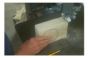
Transfer the marks for the sides of the handle to the just-cut surface.
