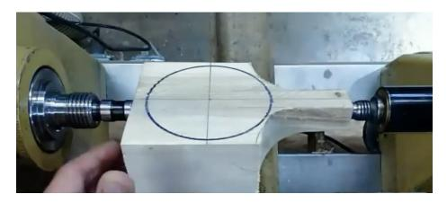
Check that your tool rest is not going to bump into the off-center cup. Carefully turn on the lathe, and bring up the speed to something comfortable (probably around 1000 RPM). Turning off-center pieces can be a bit uncomfortable, but speed does help you ride over the missing wood. Don't turn at a speed that feels too fast for you - just take your time and make steady cuts.
