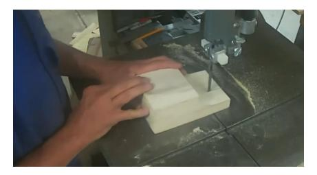
With all three cuts, leave an "arc" of extra wood between the handle and the cup, so you have enough wood to turn a transition between them.
