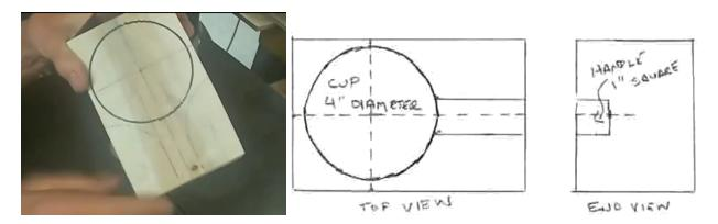
This could go right on the lathe, but there's a lot of off-center wood to remove around the handle. To cut away the excess wood around the handle on the bandsaw, transfer marks around the piece so that you can see where to cut.
