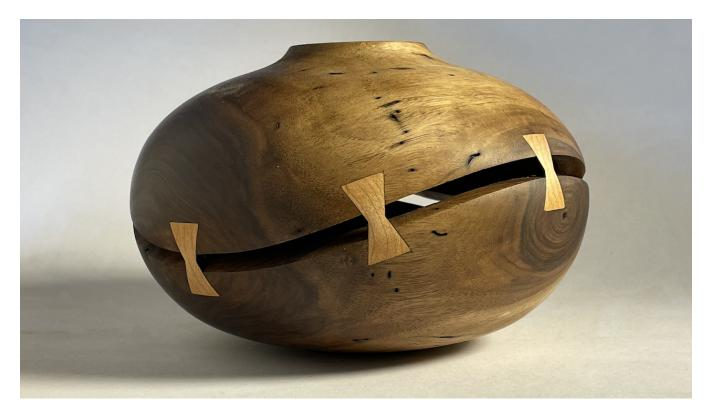
This project is relatively involved. Start with a hollow form (or a bowl or other form), remove a slice from it on the bandsaw, and reassemble the slices with pewa (butterfly patches) or similar. There are a number of steps and a special bandsaw jig is required to safely make cuts with a bandsaw.
