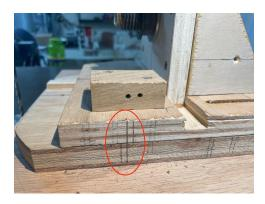
Reset the offset to the other pair of lines (cutting nearer the chuck) and make another cut.
