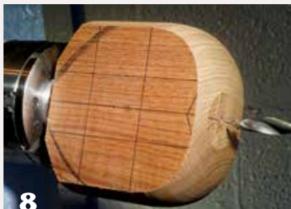
8 With the work now mounted in a chuck, the author drills into the workpiece since he wants it to serve as a dry bud vase.
