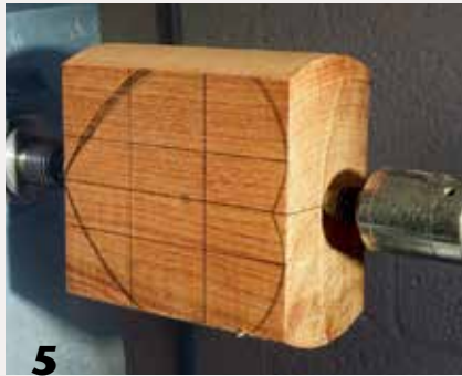
5 Since the blank is mounted in spindle orientation, with the grain running parallel to the lathe’s bed ways, it is acceptable to use a spindle roughing gouge to round the two sides.
