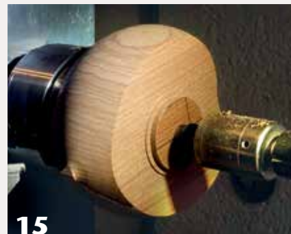
After cutting off the excess wood at the bottom tip of the heart, the author forms the first of two chucking tenons, one on each face.
