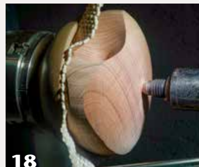
With the work jam chucked in a repurposed bowl and some drawer liner as a cushion, the author removes the tenon from the other face.
