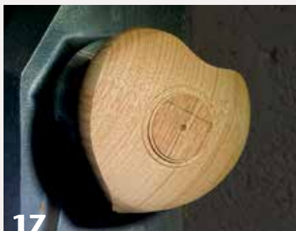
With a tenon on each side, you can continually flip the work as many times as needed to fine-tune each face, until you are satisfied with the shape of both faces. Remove one tenon.
