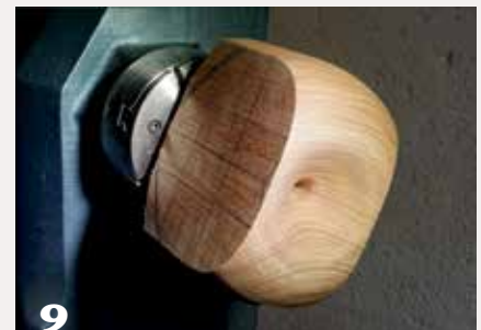
9 Carefully turn a “bowl,” or hollowed out area, at the top of the heart.
