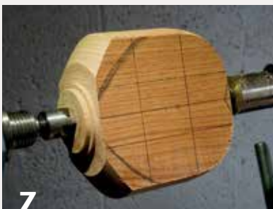
7 Form a chucking tenon at the bottom of the heart.
