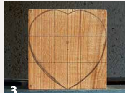
1 Accurate layout lines aid in drawing the intended heart shape as well as locating the mounting points for both axes.
