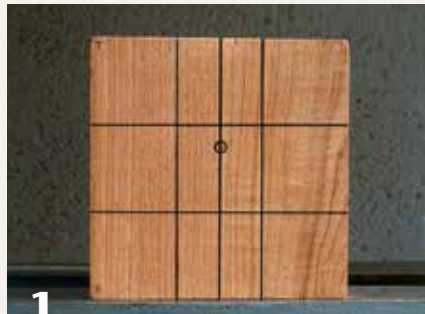
1 Accurate layout lines aid in drawing the intended heart shape as well as locating the mounting points for both axes.
