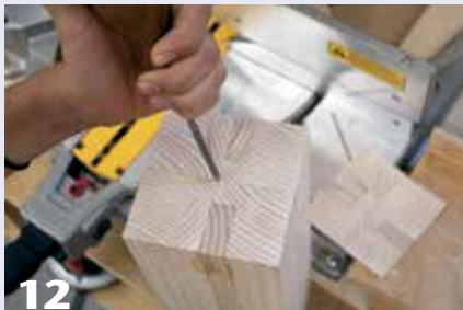
12 Prior to mounting on the lathe, mark the turning centers with a scratch awl.
