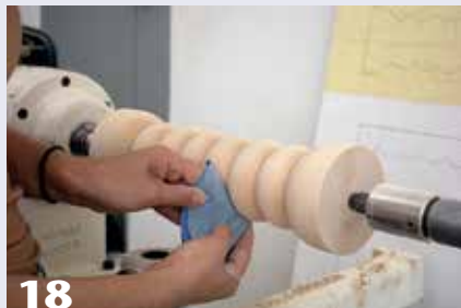
17 The author has used hide glue, so she wets the surface to raise the grain before sanding with the final grit, 320.
