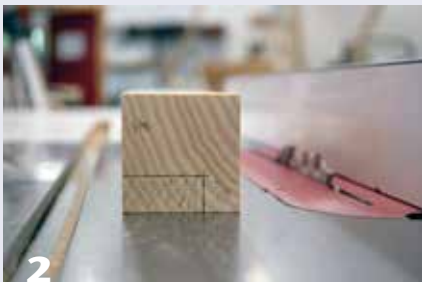
2 The rabbet at the back of the frame, which will later accept the acrylic, the picture, and the backer, is cut now, before glue-up and turning.
