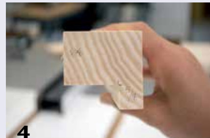
2 The rabbet at the back of the frame, which will later accept the acrylic, the picture, and the backer, is cut now, before glue-up and turning.
