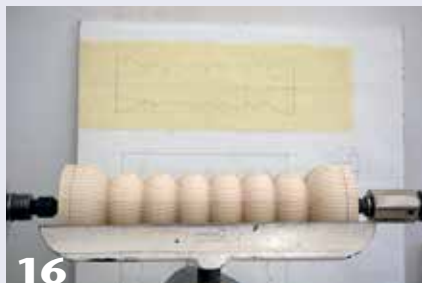
15 At the lathe, lay out and turn your desired profile. The author chooses large beads, which when stained white later will represent clouds.
