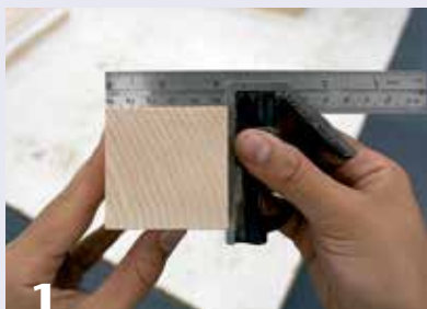
1 Each of the four quarters of this glue-up must be identical, with sides squared to one another.
