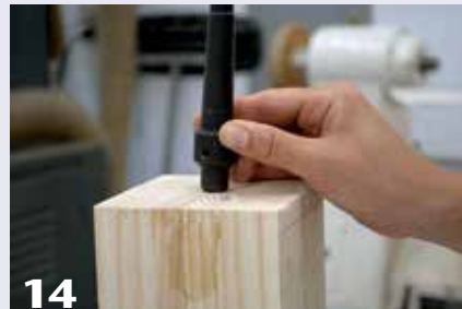
13 A cup drive center is useful, but beware the point doesn't split apart the glue-up. Either retract the point or drill a small hole to accept it.
