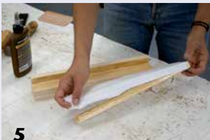
5 Use a paper glue joint to temporarily glue a waste piece into the rabbets.
