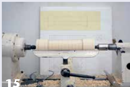
15 At the lathe, lay out and turn your desired profile. The author chooses large beads, which when stained white later will represent clouds.
