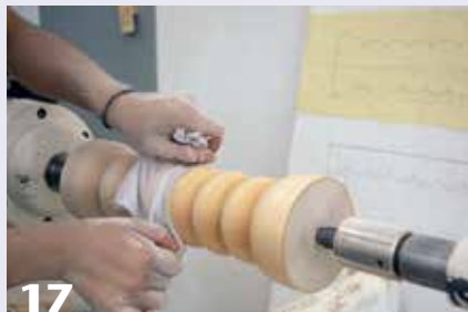
17 The author has used hide glue, so she wets the surface to raise the grain before sanding with the final grit, 320.
