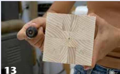
13 A cup drive center is useful, but beware the point doesn't split apart the glue-up. Either retract the point or drill a small hole to accept it.
