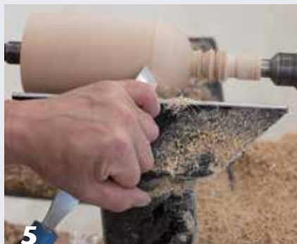
Cutting the right side of a bead with a skew. Note the three components of tool movement during the cut: vertically, upward; horizontally, from left to right; and rotationally, clockwise.
