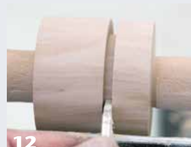
12 Parting tool cut showing some clearance on the left side of the tool after widening the cut.
