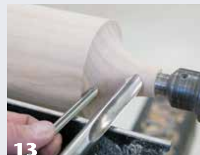
13 With relatively little mass, a ¼" (6mm) spindle gouge (at left) requires support from the toolrest close to the cutting tip. The heavier ½" (13mm) gouge is more stable and can be extended farther beyond the toolrest. Greater tool stability equates to a smoother cut.
