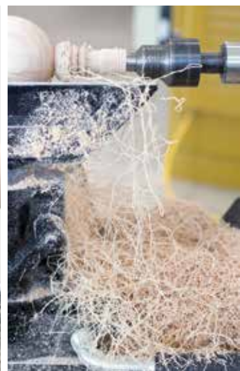
The fine "angel hair" shavings from a skew's shearing cut indicate a clean cut along the wood's sidegrain.
