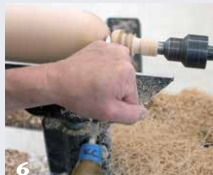
Cutting the right side of a bead with a skew. Note the three components of tool movement during the cut: vertically, upward; horizontally, from left to right; and rotationally, clockwise.
