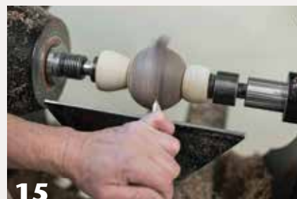
15 Before making the refining cuts, it is necessary to remove the stubs that were used to hold the piece between centers. Make sure the toolrest is far enough away for the stubs to clear. After removing the stubs, adjust the toolrest to within about 1/4" of the sphere.
