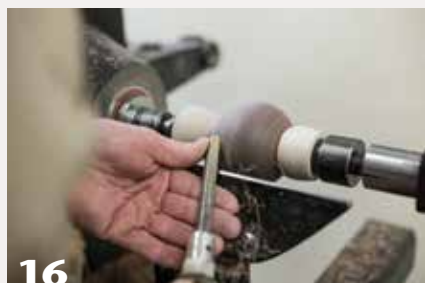
16 When the grain is oriented perpendicular to the lathe bed, make shear-scraping cuts “uphill” from small diameter to large. This allows cutting into sidegrain rather than into endgrain.
