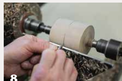
8 A clearly marked centerline serves as a reference for shaping a symmetrical sphere. Cut from the center toward each end.
