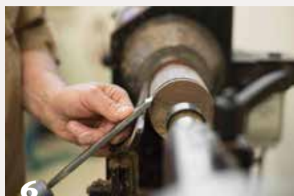
6 With the tool handle held low, the shavings do not need to change direction much as the wood is removed.
