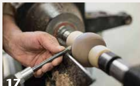
17 When the grain is oriented parallel to the lathe bed, cut “downhill” from large diameter to small, taking shearing cuts with the bevel gliding on the wood.
