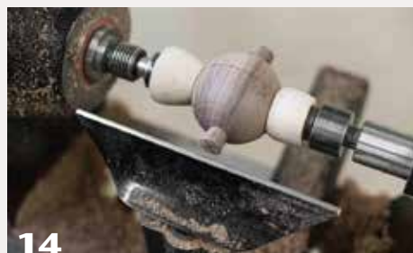
14 Cup centers allow the sphere to be rotated and mounted in any orientation, which makes it relatively easy to refine the final shape of the sphere.
