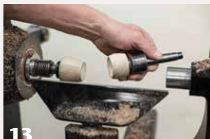
13 Cup centers are simple fixtures used for holding spheres while turning.
