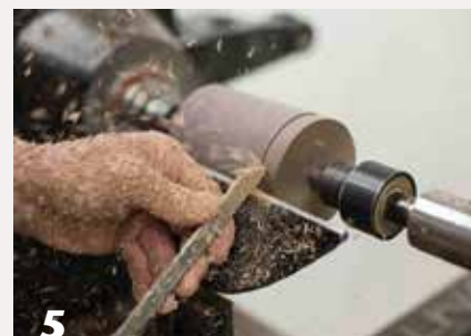
5 Begin the parting tool cut with the tool handle low to create a peeling angle. Raise the tool handle as needed while making the cut.
