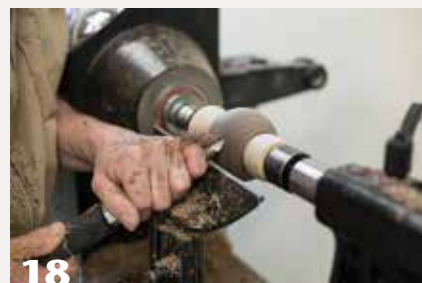
18 With the grain oriented on a bias, or askew to the lathe bed, treat the cut as if the grain is perpendicular to the bed and use a shear-scraping cut, moving “uphill” from small diameter to large.
