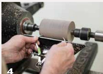
4 With outside calipers, the diameter of the cylinder can be quickly transferred to the wood to indicate the correct length of the sphere.
