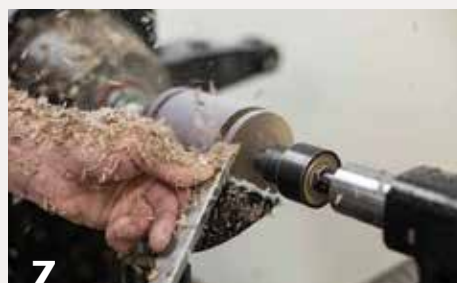
7 The peeling angle of the tool produces an efficient, clean cut.
