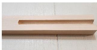
This is a handy jig for sanding the dowls. To make it, drill a 3/8 inch hole into a blank and then cut or sand the blank to expose the hole.
